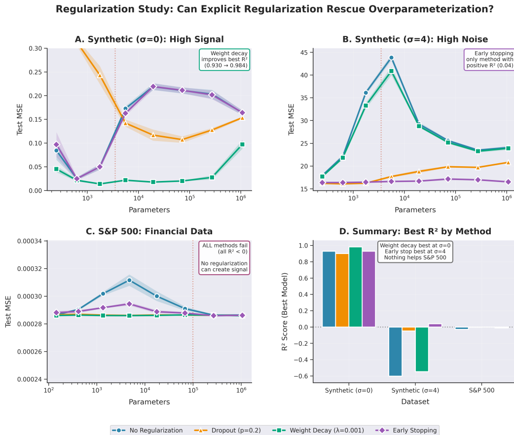
Figure 6: Regularization study across three datasets. (A) Synthetic \sigma = 0 : weight decay achieves the best performance. (B) Synthetic \sigma = 4 : early stopping is the only method with positive R^2 . (C) S&P 500: all methods produce nearly flat, overlapping curves with negative R^2 . (D) Summary of best R^2 by method across datasets.
